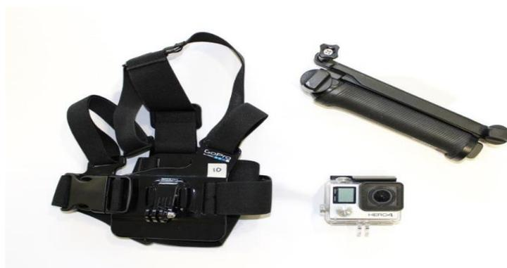
Action cameras have wide lenses to reduce their size and minimise image shake. However, such wide-angle footage may have significant perspective distortion (“fisheye effect”). This can be reduced by adjusting the camera settings during filming, or while editing the footage.
