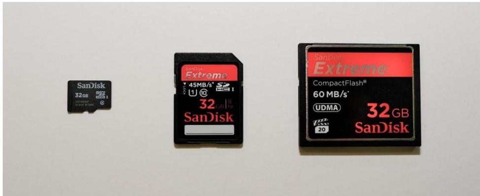
A practical starting point is to buy two cards for the camera to be used, each with the most memory that the budget allows. Once the footage has been downloaded from the card onto a computer or storage device the card should be formatted. Unlike merely deleting the images from the card, formatting ensures that all the old data has been removed and reduces the risk of data corruption and card reading errors (Carucci, 2013).
