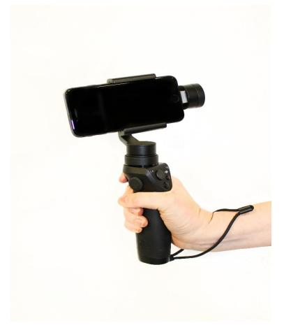
Figure 3: Smartphone mounted on a gimbal
