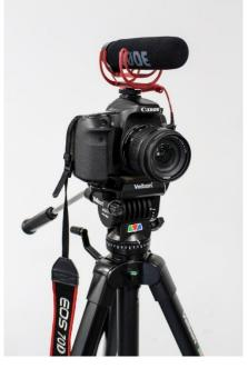
Handheld mics are not generally suitable for teaching videos as they tend to distract both the person in front of the camera and the viewer. Boom mics can be either attached to the camera (Figure 4) or held overhead and just out of shot on a pole. The latter requires an additional person to assist with filming. Small boom mics that attach to the camera and plug into the
